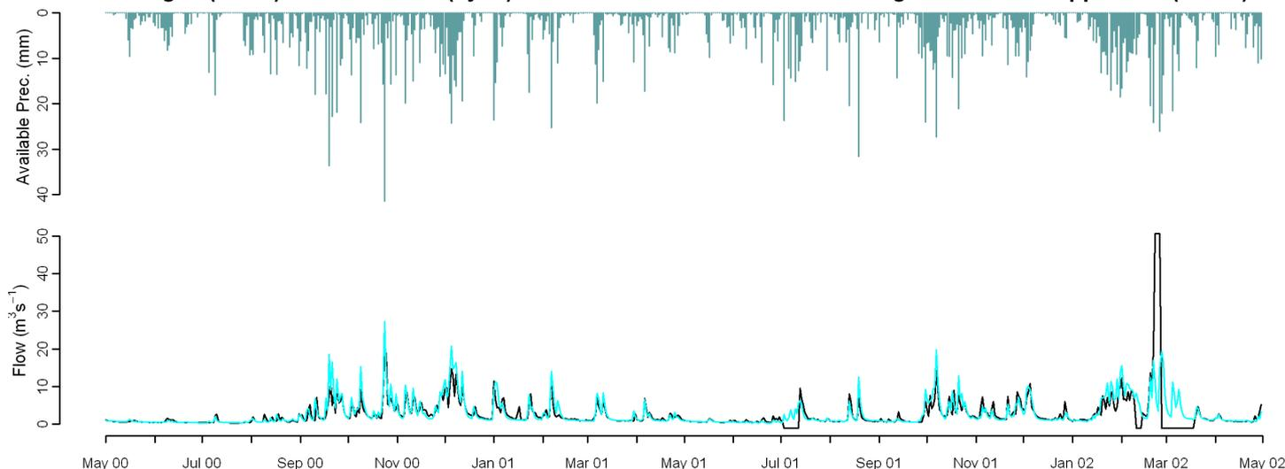
Comparison of gauged and simulated flow (observed and modelled climate)
