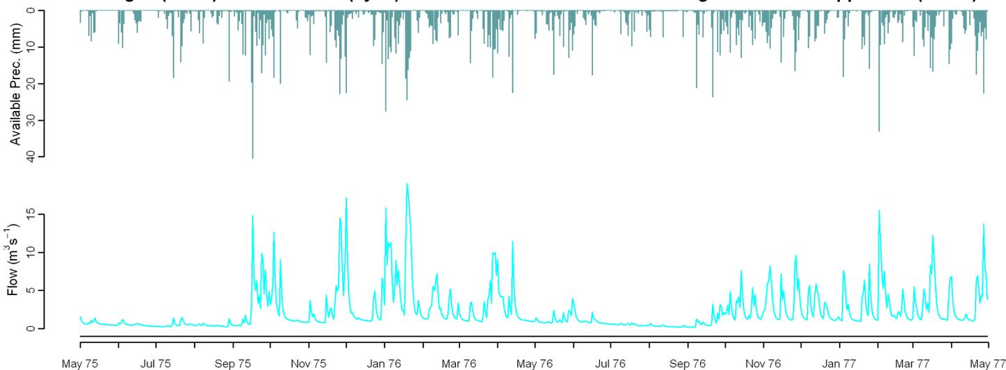
Gauged (black) and simulated (cyan) flows from observed climate - Douglas Water at Happendon (84037)
