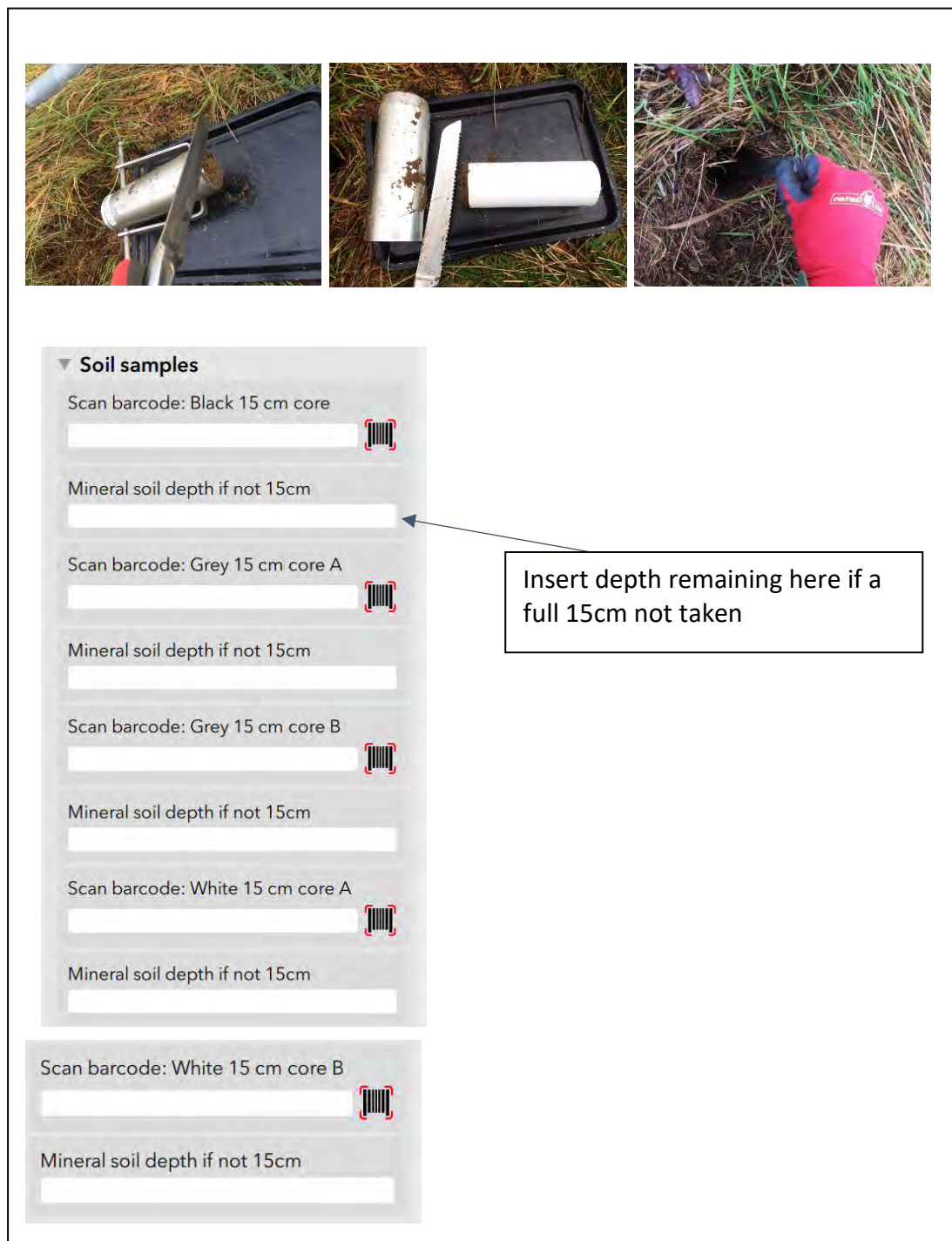
Figure 10. – Trim the core and measure the depth of hole if needed. If the core didn't fully penetrate to 15cm, record the depth from the bottom of the cross bar to the ground surface in the software and take a "short" note on the plastic bag. This is so we can work out the correct bulk density and do not mistake it with a compressed ("comp") core.
