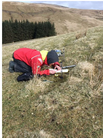
© Photos by S. Reinsch: Soil water infiltration measurements at Newborough Warren (left), Plynlimon (middle) and Wymondham (strawberry field) in spring 2018.
