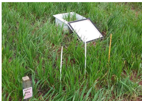
© Photos by A. Carswell (left) and A.R Sánchez-Rodríguez (right): Static N 2 O chamber at North Wyke (left) and automated N 2 O chamber at Henfaes farm (right).
