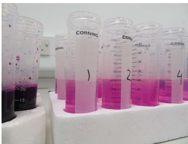
© Photos by S. Reinsch: Colorimetric measurement of permanganate oxidisable C from soils.
