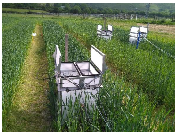
© Photos by A. Carswell (left) and A.R Sánchez-Rodríguez (right): Static N 2 O chamber at North Wyke (left) and automated N 2 O chamber at Henfaes farm (right).
