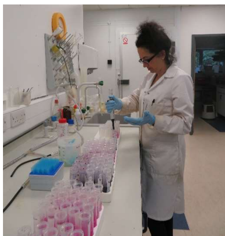
© Photos by S. Reinsch: Colorimetric measurement of permanganate oxidisable C from soils.
