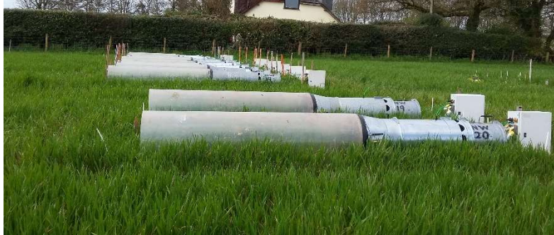
© Picture by A. Carswell: Wind tunnels for measuring ammonia emissions on winter wheat at North Wyke.
