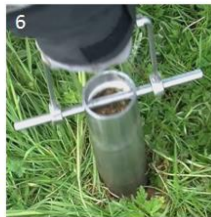
6 Remove from soil, extract core, cap, red at top, black at bottom, bag
