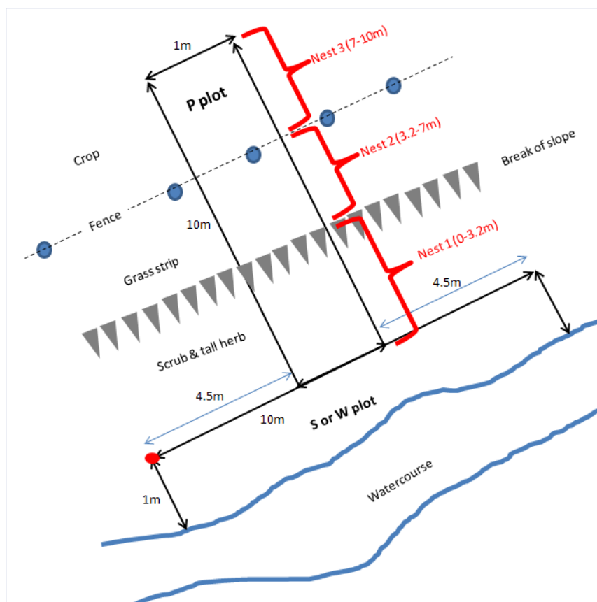
Figure 5.11.1: Layout of P plot. The red blob shows the location of the differential GPS point for the S or W plot. The nest lengths here are an example only. In reality the number of nests and their sizes will vary at the surveyor's discretion up to a total of 6 nests i.e. from 0 to 5 as for the X plots.
