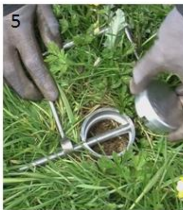
5 Knock coring device in until cross bar is flat on surface
