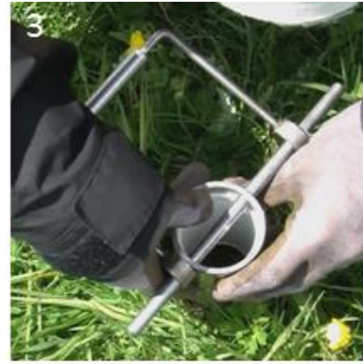
3 Place plastic core in coring device
