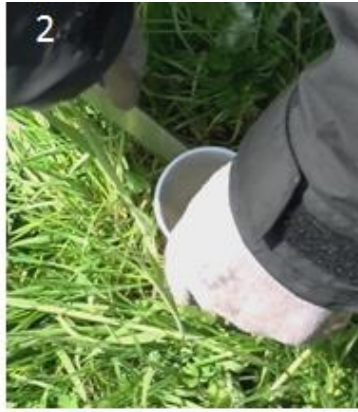
2 Use knife to cut roots around core
