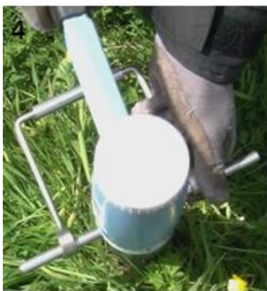
4 Knock coring device into soil
