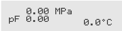
This is the main menu, displaying the water potential in both MegaPascals (MPa) and pF, and the sample temperature in °C.
