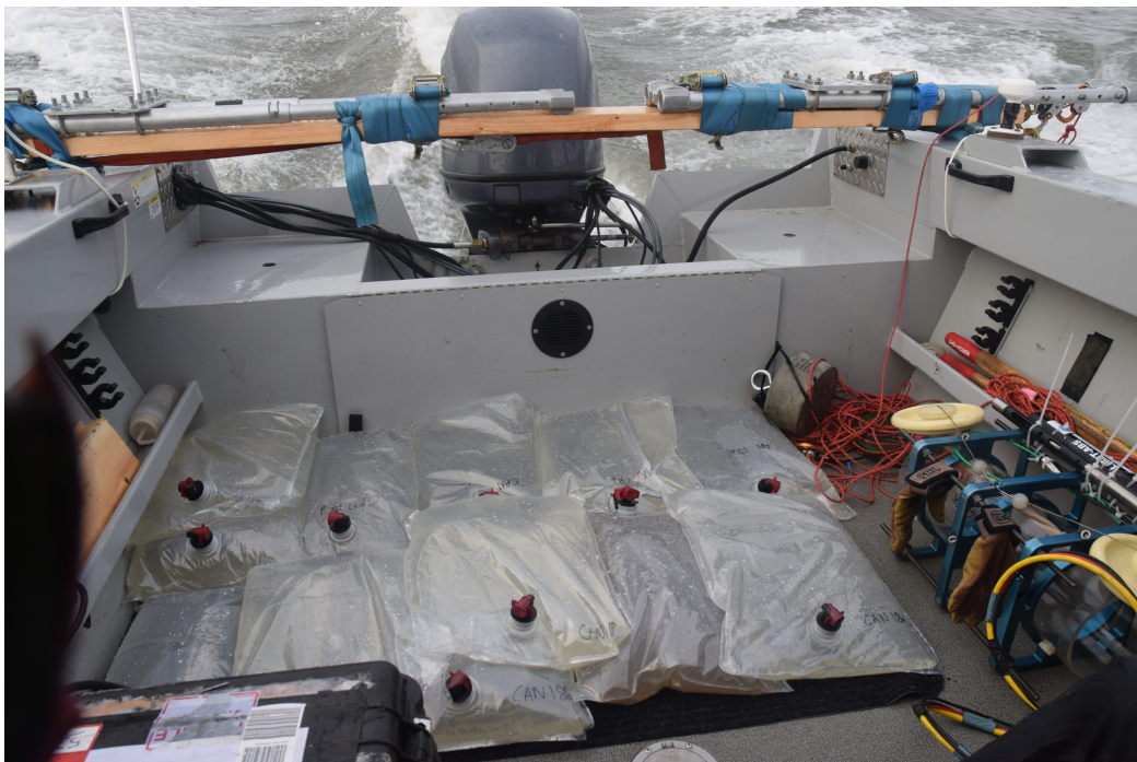
Figure 2: Samples collected from varying depths in the Mackenzie Estuary. The modified Van Dorn™ depth sampler and attached salinity probe are shown to the right of the samples.
