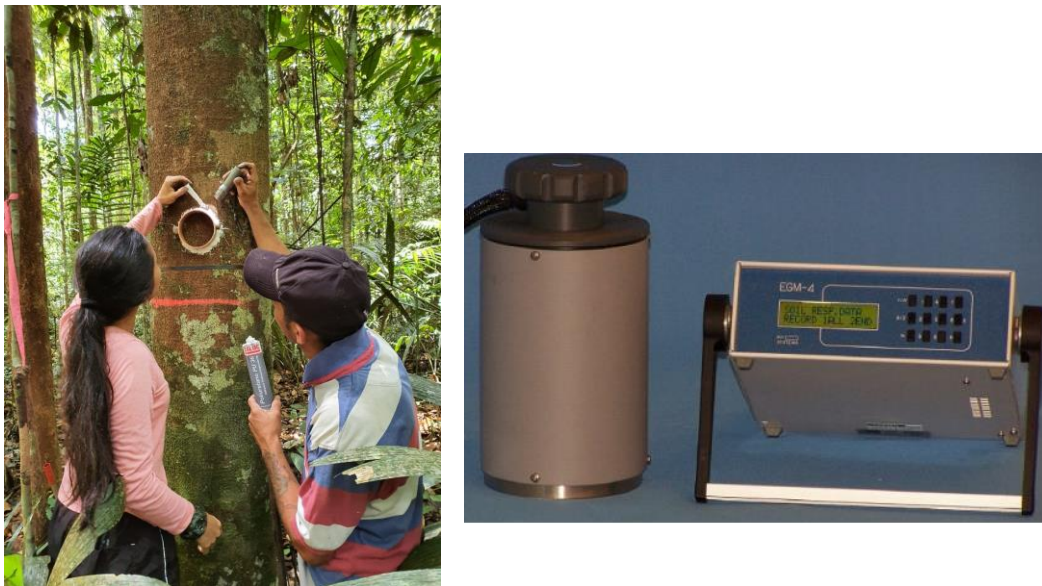
Figure 3: A) The collar was sealed with a special glue, and inspections with a flashlight were made to check for any holes B) An EGM-4 portable Infra Red Gas Analyser (IRGA) right and the chamber (left) for measurement of CO 2 efflux.
